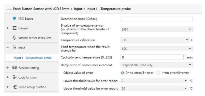
Fig. 5.4.1 Parameter setting of temperature probe
