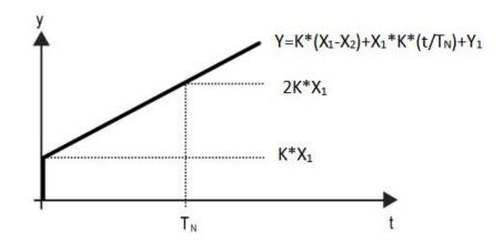
Fig.5.5.2 (3) control value of PI control mode
