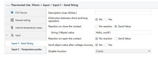
Fig.5.4.2(3) Parameter setting of sending sting
