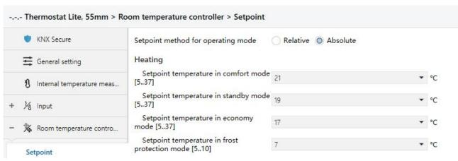
Parameter setting of absolute adjustment (2) Fig.5.5.2.1.1 "Setpoint" parameter window
