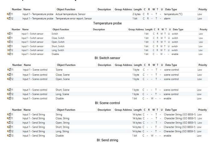
Fig.6.3 "Input" communication object
