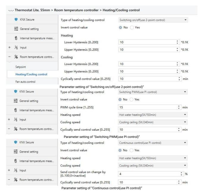
Fig.5.5.2.1.2(1) "Heating/Cooling control" parameter window
