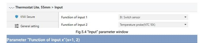
This parameter is for setting the function of external input interface. Support temperature detection and dry contact input (BI), setting page will be visible when select corresponding chosen. Also can be disable this channel function. Options:
