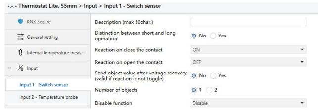
Fig.5.4.2(1) Parameter setting of switch sensor
