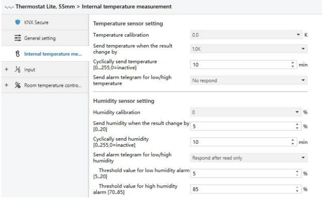
Fig. 5.3 "Internal sensor measurement" parameter window
