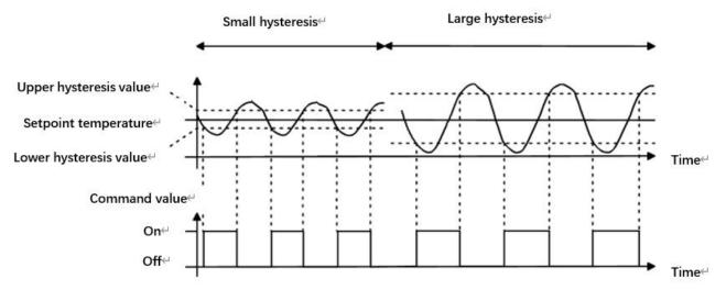
Fig. 5.5.2 (2) Effects of hysteresis on control value switch action(heating) under2-point control mode
