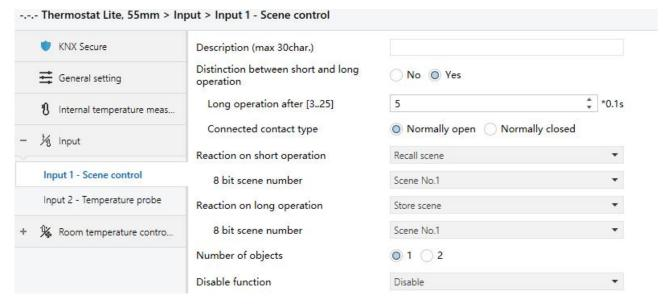
Fig.5.4.2(2) Parameter setting of scene control
