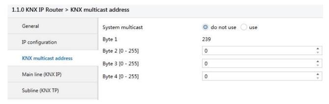
Fig. 4.4: KNX multicast address
