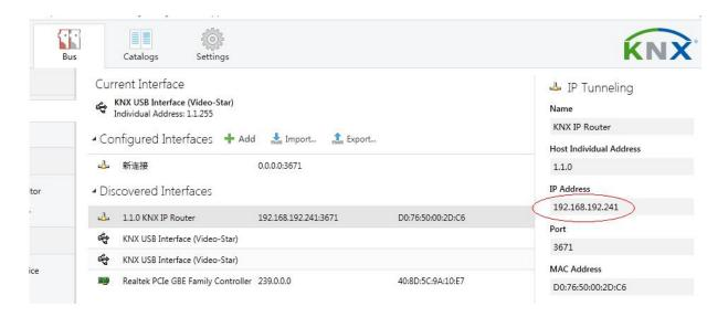
Fig. 5.2: Identifying IP address with ETS
