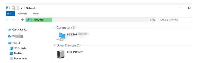
Fig. 5.1: as UPnP network device (KNX IP Router)
