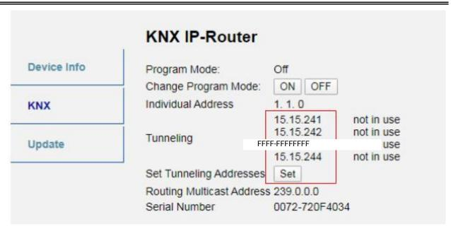
Fig. 5.11: Additional Tunneling Address Assignment in the Web Front-end
