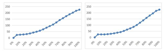
Fig.3: 2 exponent dimming curve
