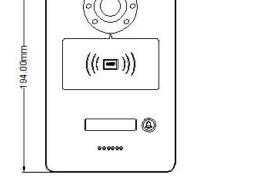
Suggested Installation Height: camera is 1.6m above the ground
