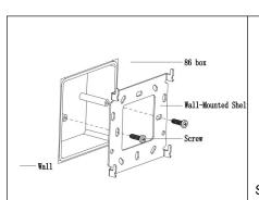
Step 1: Aim the screw hold of bracket with the holes of 86 box. Tighten the screw and fix the bracket.
