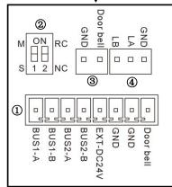
BUS1-A BUS1-B: Bus Interface 1; BUS2-A BUS2-B: Bus Interface 2;
