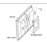
Step 2: Connect the indoor monitor with wire, and aim the slot with the hanger of bracket. Then, move down the device a little bit. It's fixed when hearing the sound of joint.
