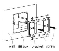
Step 3: Align the card slot with hanger hole.
