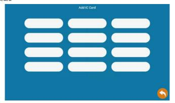
Register a new card by swiping it at the swipe area of Outdoor Station, in the meantime a card number appears in the blank box on Indoor Monitor. Then a new card is successfully registered. Repeat the operation to complete registration of multiple cards. 12 cards can be added maximum.
