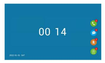
**Standby Interface:** unread calls, unread messages, unread motion detection and unread camera records are available in the bottom right corner of the screen.
