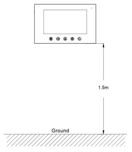
Recommended installation height: 1.5m from ground at the bottom of the device
