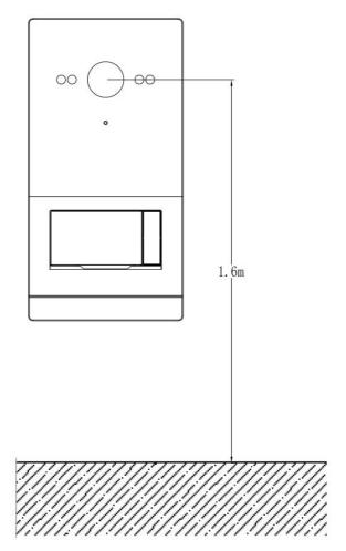
Suggested Installation Height: camera is 1.6m above the ground
