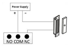
Wiring for normally closed type lock(Magnetic Lock)
