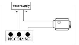
Wiring for normally open type lock(Electronic lock)
