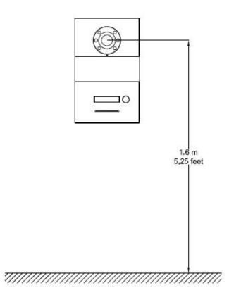
Recommended Installation Height: camera is 1.6m above the ground
